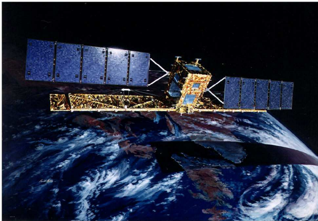
CSA illustration of the Radarsat Satellite. The SAR antenna shown in gold beneath the satellite is 15 m long and 1.5 m wide.
